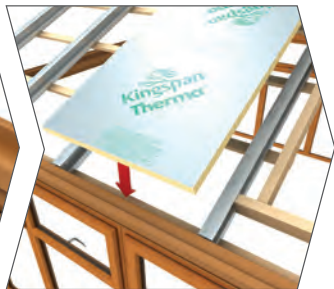
Install external insulation
