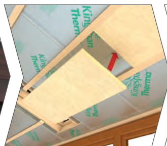
Install insulation between batten
